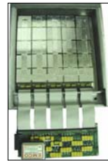
Figure 2. A 5 module x 5 module CZT detector and associated electronics. The detector is shown with the collimator removed. Each module is 2.54 cm x 2.54 cm.
